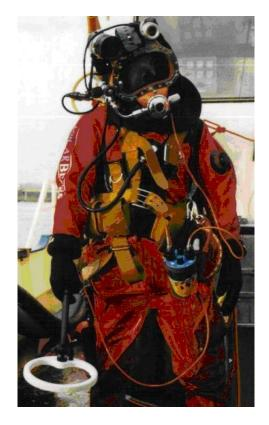
Diver prepared for EOD survey using AQ1B-Compact/20cm - Harness mounted
