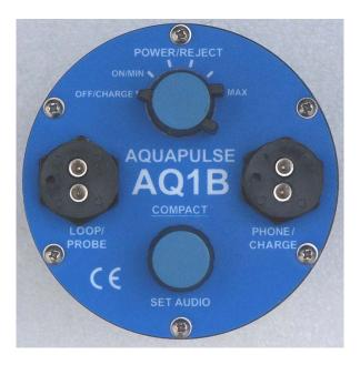
The **Aquapulse 1B-Compact** underwater metal detector is a precision built instrument using the latest pulse induction techniques, and has been designed for both ease and simplicity of use in the underwater environment, featuring good detection performance for locating both ferrous and non-ferrous metals.
