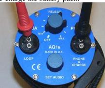
Battery Test Points (shown on the Standard AQ1B)
