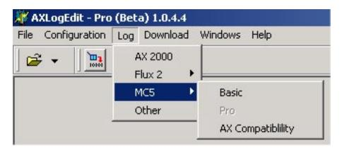
MC5 "**Basic**" is for an MC5 Magnetometer without the optional NMEA interface and combiner circuitry. This will log only the deviations.
