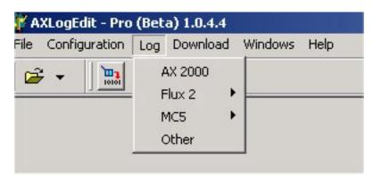
Select "**AX2000**" if logging from an AX2000 Magnetometer or select "**MC5**" if logging from an MC5 Magnetometer. If "**MC5**" is selected, three additional selections will appear to identify the MC5 configuration as shown below:
