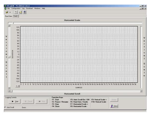
This screen allows the user to see the data in graphic format as it is logged. This is a very powerful display function that allows the user to vary both the vertical and horizontal scales.
