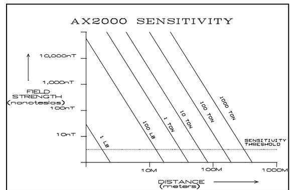
By taking the maximum sensing distance for a given target and producing a simple scale diagram - the optimum search lane width can be derived. The procedure is as follows: -
