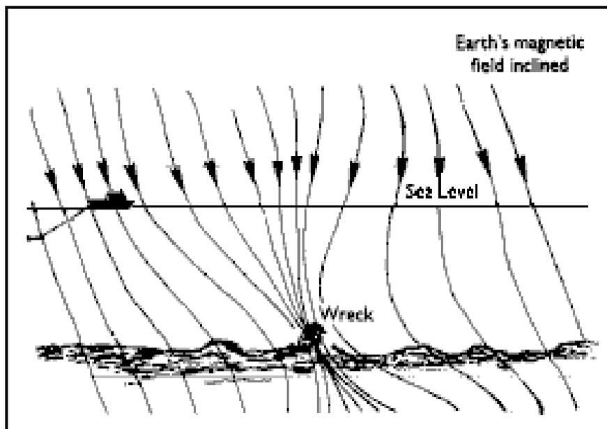
*THE MAGNETIC INFLUENCE OF A WRECK CAN BE DETECTED AT DISTANCES EXCEEDING 400M*
