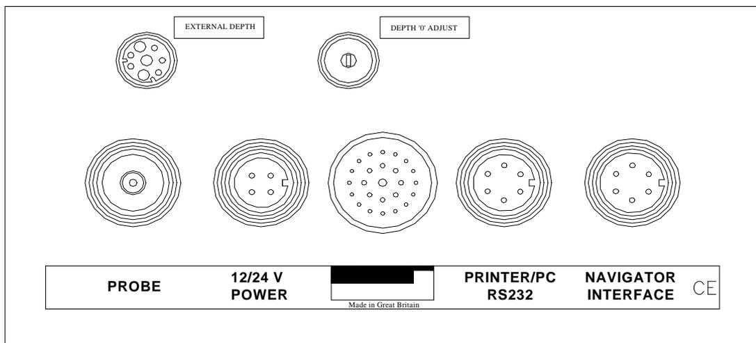
**PROBE** - The *Toroid* probe is connected via connects to the AX2000 via the dedicated waterproof phono connector.
