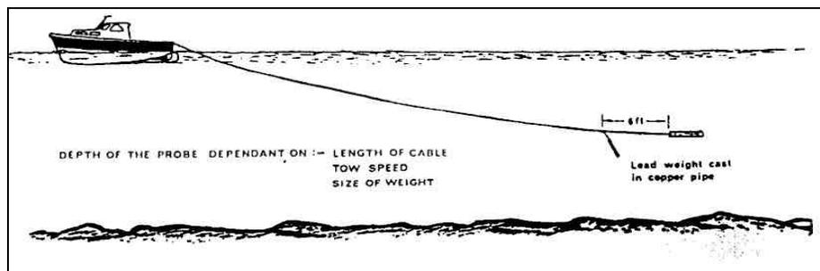
In cases where the object to be detected is at a depth that would not allow positive detection with the tow-fish at the surface, requires that the tow-fish be deployed at a height above bottom that would guarantee a response within the search parameters employed. The use of a lead ballast weight close to the tow-fish, is a simple but effective method of achieving increased tow-fish depth for a given speed.
