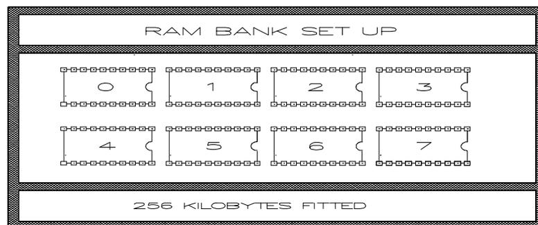
The above display confirms the extended 256Kbyte RAM configuration is fitted; each position is occupied and is equivalent to 32Kbyte. In the case of the AX2000 PES & PET this equates to 8 x 32 i.e. 256Kbyte, this is the maximum capability, and allows a data-logging storage time of approximately 10hrs duration.
