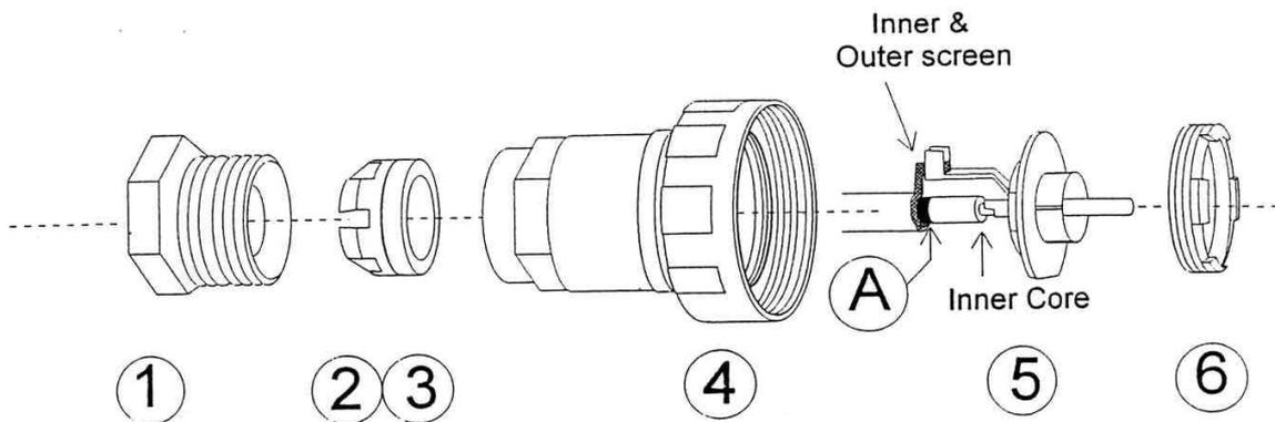
(A) Anti-phonic semi conductor black layer cut back
