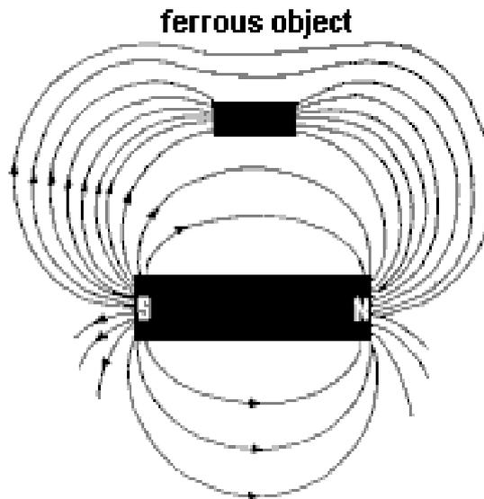
*THE MAGNETIC ANOMALY OF A FERROUS OBJECT IN A UNIFORM MAGNETIC FIELD*
